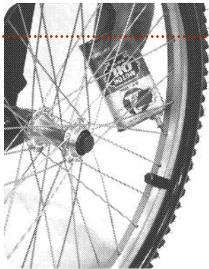
Spokes Put a tiny drop on each spoke where it enters the nipple.
