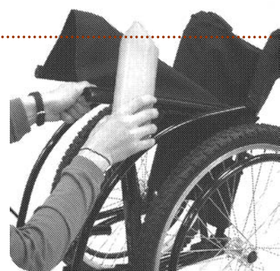
Seat tubes and side frame When chair is folded, rub candle wax onto the contact surfaces between seat tubes and side frame. The wax will make folding easier and prevent the paint scraping off.
